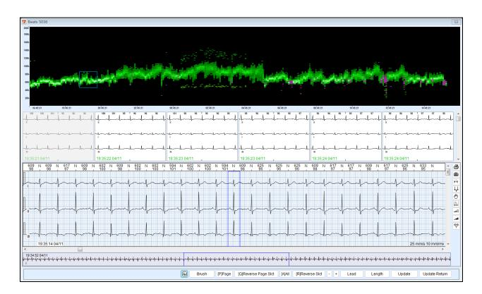
On the top is the RR bird view where the X-axis indicates time and Y-axis indicates RR interval. RR intervals are sorted by colors. Green indicates normal, red indicates VE, and purple indicates SVE. This histogram contains the following operations:
