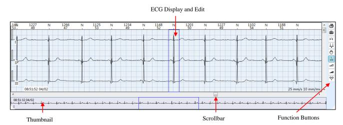
The ECG view window consists of the ECG display/edit area, thumbnail, and function buttons.
